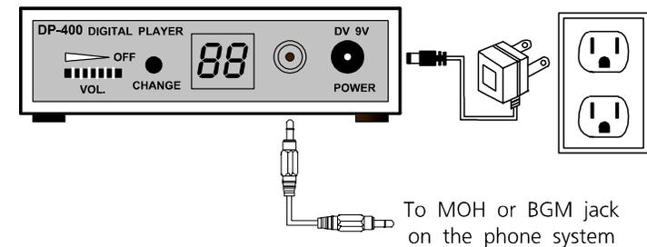
Connect the power supply and the audio patch cord. Two different audio patch cords are provided. Use the one that fits your phone system.
