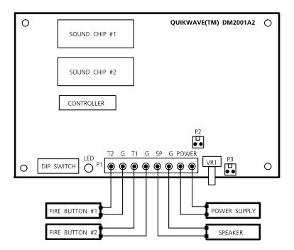
The EM2001A is a highly reliable digital sound box designed for use in coin operated kiddie rides and other equipment where a continuous sound loop needs to be played.
