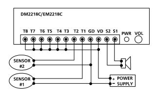
Normally closed switches and sensors are often used in security systems.
