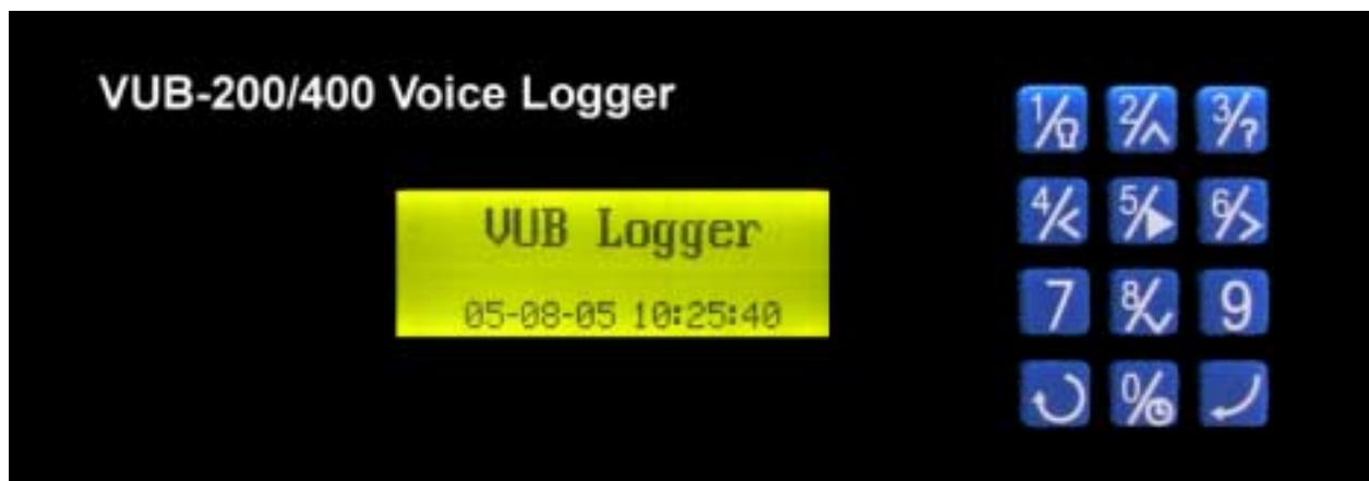
VUB Logger front view, showing speaker, LCD display and keypad.
