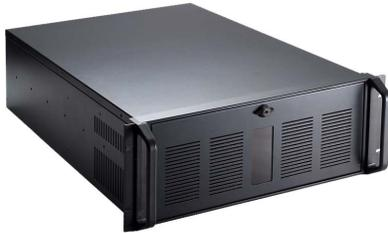
eALog is an open platform voice logger built with cutting edge technologies. It is capable of passively tapping into digital or analog phone lines for real-time call recording and/or monitoring without any noticeable interruption in the service. Recordings are stored internally and can be retrieved locally or remotely via telephone or LAN. eALog can be purchased as a turnkey system complete with application software, or with SDK (software development kit) for building your own system.
