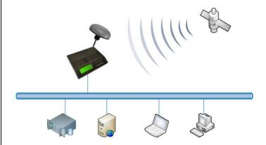
The NTP-100 Time Server is designed to provide very accurate time obtained from GPS satellites, so that all PCs in the same network can be precisely synchronized without accessing any outside NTP servers.
