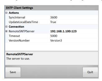
**SyncInterval:** The time synchronization interval between the PC and the NTP100. Default is 3600 second (1 hour), minimum setting is 1 second.
